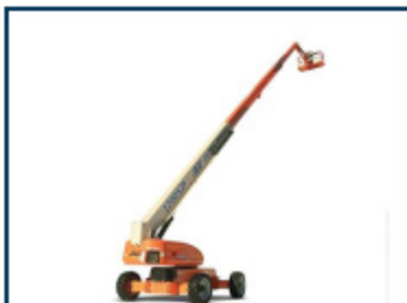
BOOM LIFT / MAN LIFT
